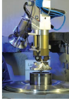
Forged-milled compressor wheel production
