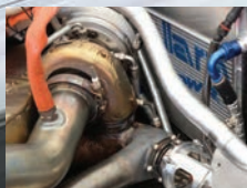
Twin EFR-7163 turbochargers used to boost the Verizon IndyCar® Series.
